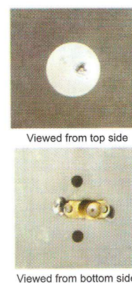
Figure 5: First DGS-integrated antenna explored to suppress cross-polarized radiations.
