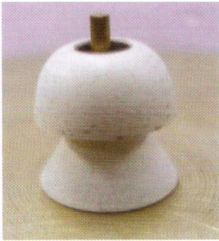
Figure 9: Pawn shaped dielectric ring surrounding a vertical monopole: a UWB design.
